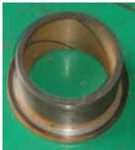
**Application field** Two-layer anti-friction products, manufactured with the use of developed antifriction material, modified by nanostructured particles in the form of oxide components, technologies and equipment are used in friction tribotechnical purpose machines and mechanisms operating in the regime of intense abrasive wear.
