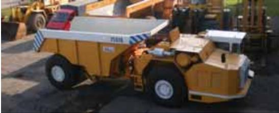
**Application field** The underground dump truck is intended for transportation of muck and minerals on routes of underground mine openings with a length to 8 km and average slopes to 12 %. The maximum level of mine water on separate parts of a route may be to 1 m.
