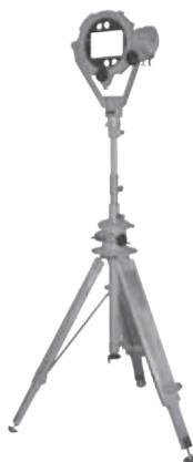
Azimuthal mechanism is arm installation azimuthal angle and smooth height adjustment, locking screws azimuth mechanism and height. The zeros of the reference azimuth are set by turning the pointer on a limb mechanism and the rotation of the Vernier drum on the axis of the worm.
