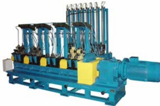
**Machine for torque breakdown test of grinding wheels SR-400V**
