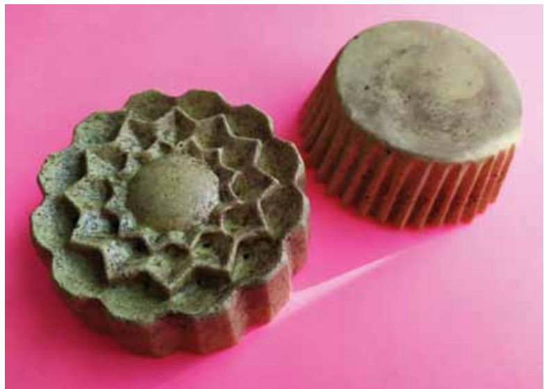
Samples of sulfur concrete
