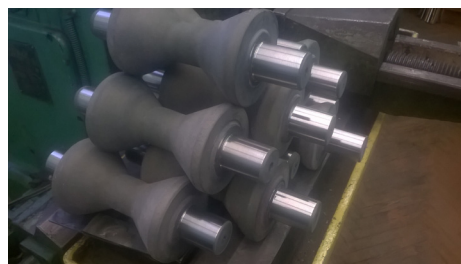
WIRE DRAWING ROLLERS, HARDENED BY GAS FLAME SPRAYING
