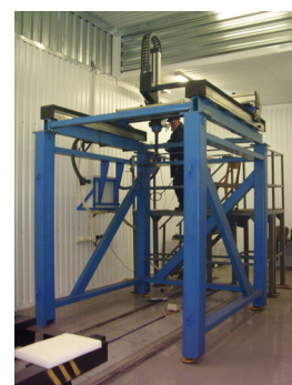
INSTALLATION OF LASER THERMAL HARDENING OF LARGE-SIZED PARTS (OJSC “BELAZ”)
