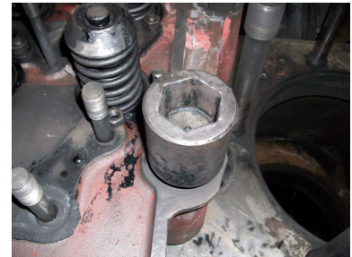
THREADED CONNECTIONS FASTENING THE CYLINDER HEADS OF DIESEL ENGINES OF DIESEL LOCOMOTIVES CHME-3
