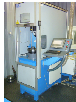
INSTALLATION OF LASER THERMAL HARDENING OF SMALL-SIZED PARTS (OJSC “BELAZ”)
