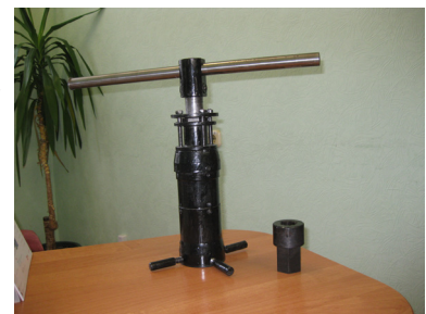
BALLOON WRENCH WITH INTERMEDIATE ROLLING BODIES
