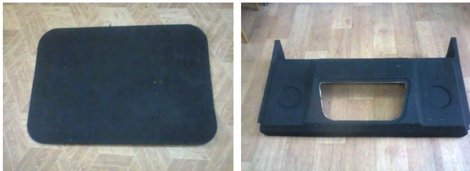
WPC ceiling sheet and detail (cab of MTW tractor)
