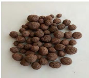
*Thermal insulating porous filler*
