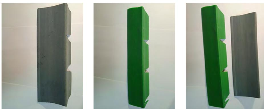
Packaging polymer material modified with SiC nanoparticles for building blocks
