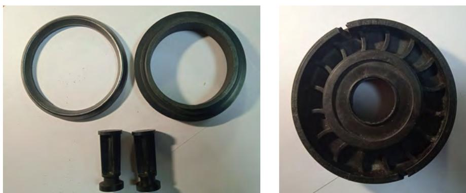
Products made from polymer materials containing graphene particles
