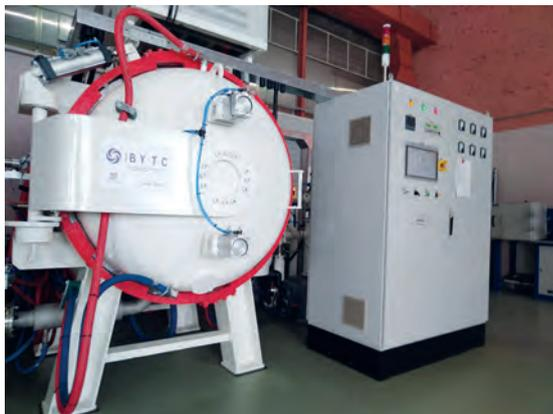
Equipment for sintering carbide blades
