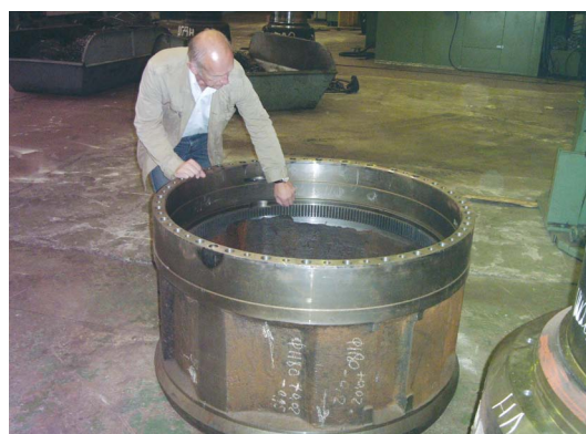
Assessment of the quality of hardening of a part of BELAZ OJSC
