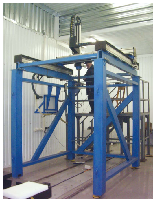
Installation of laser thermal hardening of large-sized parts of BELAZ OJSC
