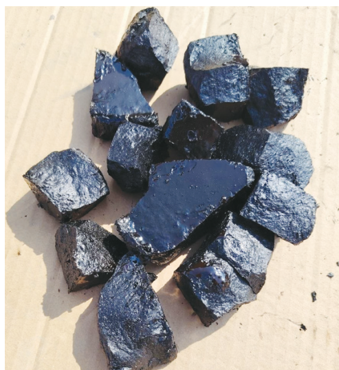
The waste from the plant is solid carbon residue (Pitch)
