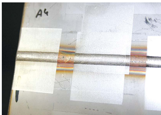
Laser cleaning process of the weld
