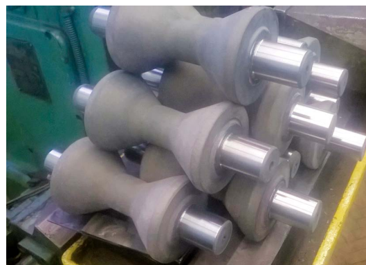
Wire drawing rollers, hardened by gas flame spraying
